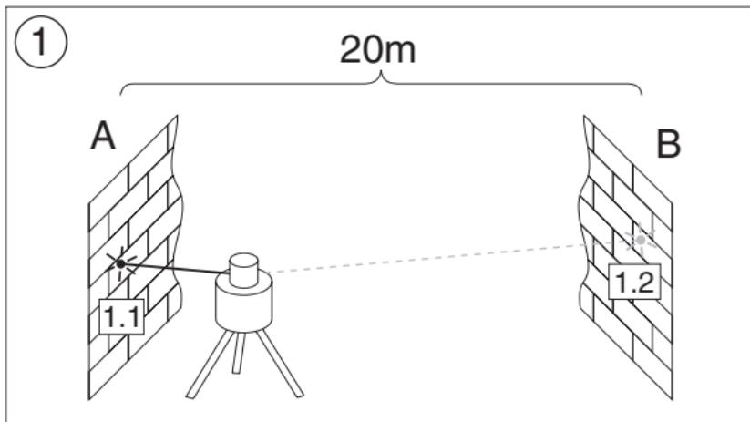
Now, place the unit near wall B., with the X-axis pointing towards wall B. After the unit is level, mark the height of the laser spot at the centre of the beam at wall B. Turn the entire unit 180°, let it self-level and mark the center of the laser spot at wall A. The difference (h) of the marked points at wall A shows the deviation.
